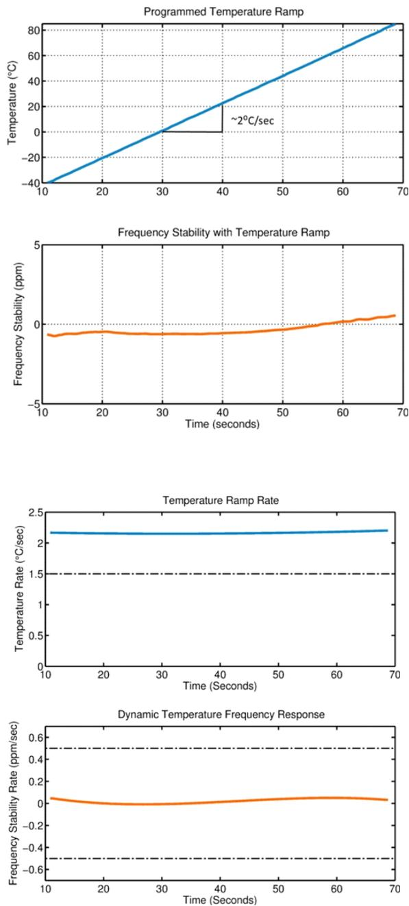
Frequency accuracy under a moderate temperature ramp up to 2°C/sec is limited by the TC-MO's trimmed accuracy of the frequency stability over-temperature.
