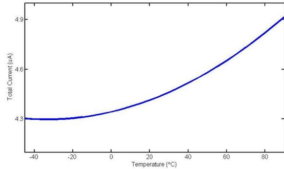
Figure 4. Supply Current over Temperature (No Load)
