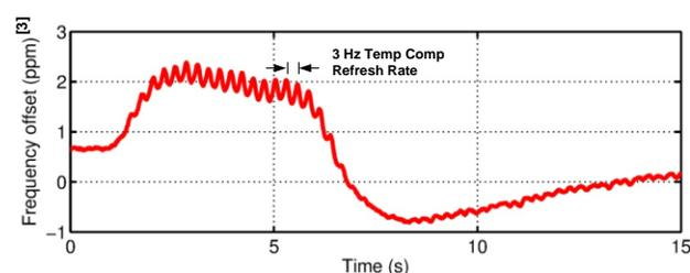
For temperature ramps  $>5^\circ\text{C}/\text{sec}$ , the frequency accuracy is limited by the update rate of the temperature compensation path (see the  $5^\circ\text{C}/\text{sec}$  and  $10^\circ\text{C}/\text{sec}$  plots).
