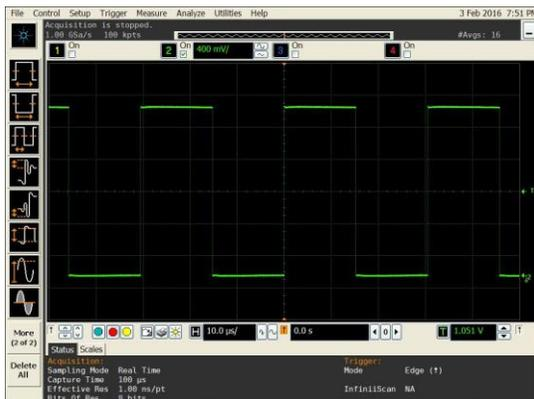
Figure 7. LVCMOS Output Swing
