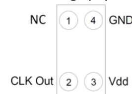
**Figure 1. Pin Assignment**
