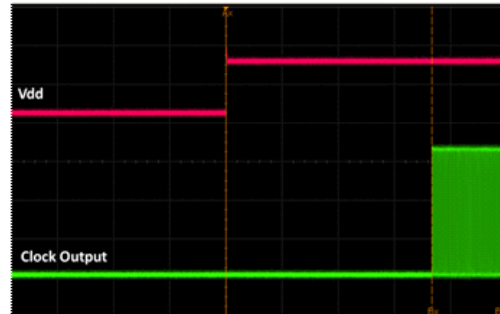
Figure 17. Startup Waveform vs. Vdd
