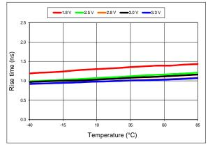
Figure 12. 20%-80% Rise Time vs Temperature
