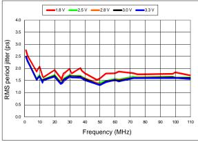
Figure 10. RMS Period Jitter vs Frequency
