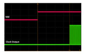
Figure 17. Startup Waveform vs. Vdd
