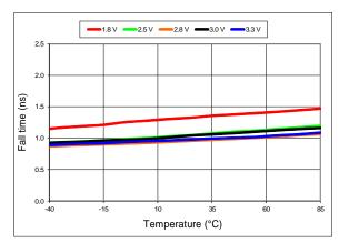
Figure 13. 20%-80% Fall Time vs Temperature
