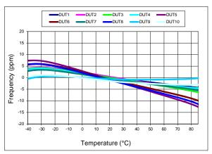
Figure 9. Frequency vs Temperature
