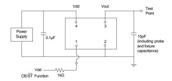
Figure 2. Test Circuit
