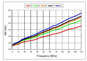
Figure 8. Idd vs Frequency
