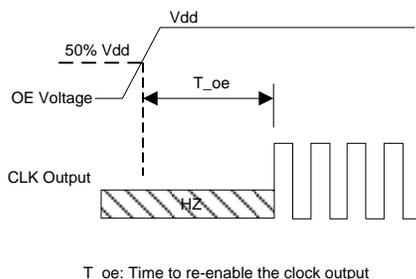
T\_oe: Time to re-enable the clock output
