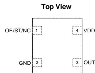
**Figure 1. Pin Assignments**
