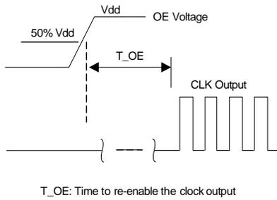
**Figure 6. OE Enable Timing (OE Mode Only)**
