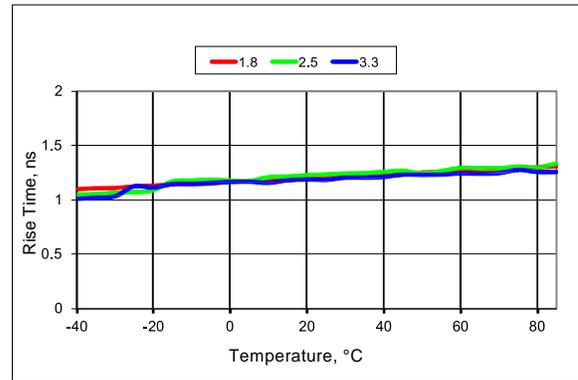
Figure 13. Rise Time vs Temperature, 75 MHz Output 10%-90% Vdd
