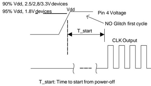
**Figure 4. Startup Timing (OE/ST Mode)**
