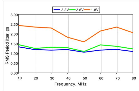
Figure 9. RMS Period Jitter vs Frequency
