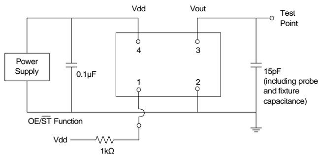
**Figure 2. Test Circuit**
