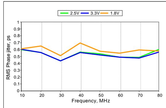
Figure 11. RMS Phase Jitter vs Frequency
