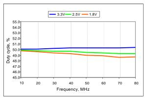
Figure 10. Duty Cycle vs Frequency
