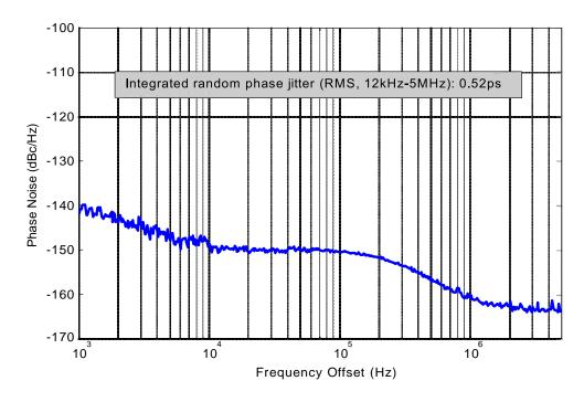
Figure 1. Phase Noise, 10 MHz, +3.3V, LVCMOS Output
