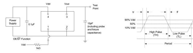
Figure 2. Test Circuit
