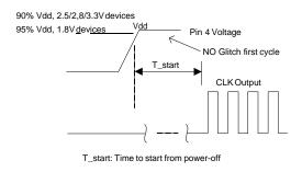
Figure 4. Startup Timing (OE/STMode)
