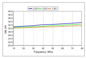
Figure 8. Idd vs Frequency
