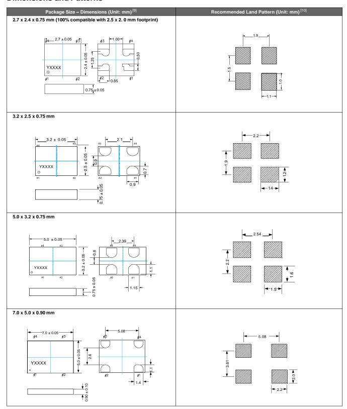
9. Top marking: Y denotes manufacturing origin and XXXX denotes manufacturing lot number. The value of "Y" will depend on the assembly location of the device.
