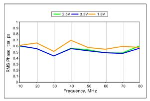
Figure 11. RMS Phase Jitter vs Frequency
