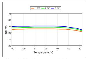
Figure 12. Idd vs Temperature, 10 MHz Output
