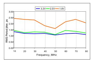
Figure 9. RMS Period Jitter vs Frequency
