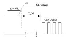
T\_OE: Time to re-enable the clock output
