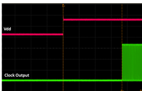
Figure 17. Startup Waveform vs. Vdd
