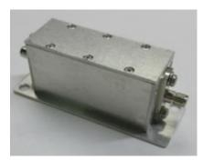
A crystal filter that is inserted between the antenna and the radio. Achieves removal of interfering frequencies near the own frequency and reduction of spurious due to non-linear distortion.
