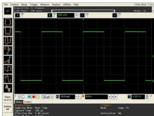
**Figure 9. LVCMOS Output Swing**
