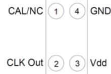
**Figure 1. Pin Assignment**
