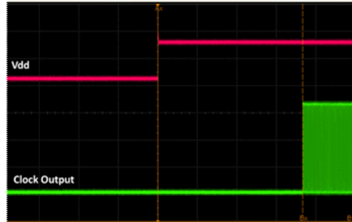
Figure 17. Startup Waveform vs. Vdd
