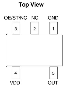
**Figure 1. Pin Assignments**
