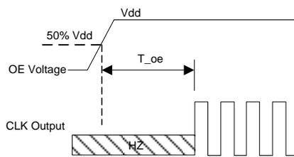
T\_oe: Time to re-enable the clock output
