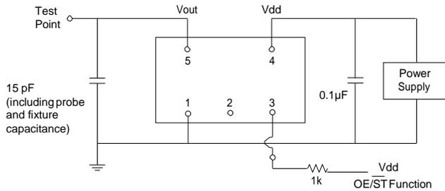
**Figure 2. Test Circuit**
