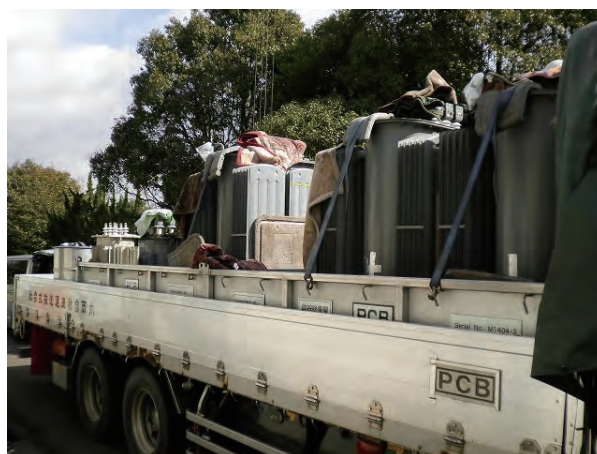
Low-concentration PCB waste is being transferred onto a specialized waste transport vehicle of a disposal company
